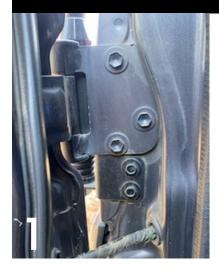
FOR REFERENCE THE IMAGE 1 IS OF A BRACKET INSTALLED AND IMAGE 2 IS OF NO BRACKET INSTALLED
